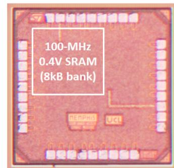
Figure 2: Die microphotograph of the MEMPHIS prototype in 28 nm FDSOI CMOS.
