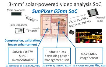
Figure 1: SunPixer SoC in 65nm CMOS.
