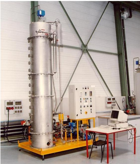
**Figure 1: Picture of a tubular reactor (fixed-bed reactor for anaerobic digestion).**
