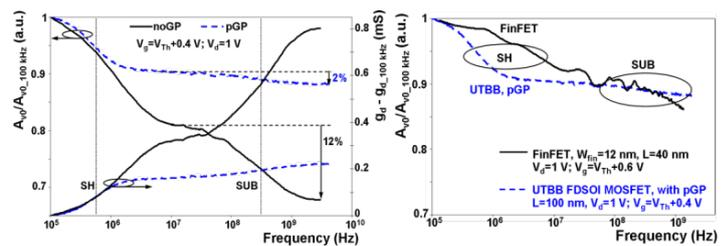
Figure 2: GP effect on  $g_d$  and  $A_{vo}$ .  $L=100$  nm.  $W=30$  μm.  $T_{box}=10$  nm (left).  $A_{vo}$  vs frequency in UTBB MOSFETs and FinFETs [1] (right).
