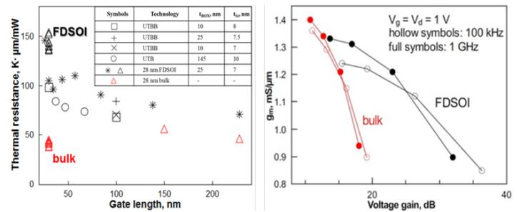
Figure 1: Thermal resistance in devices from various technologies (left).  $g_m$  vs.  $A_{vo}$  in bulk and FDSOI devices (right) [5].
