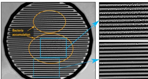
Figure 1: Concentration of bacterial cells on the capacitive sensor thanks to AC-electroosmosis.
