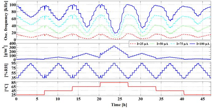
Figure 2: Oscillation frequency variations under different temperature and humidity levels and 4 different input currents.
