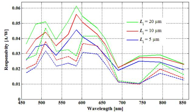
Figure 3: Measured typical responsivities versus light wavelength for the on-membrane (solid curves) and on-substrate (dashed curves) photodiodes ( $L_i = 5/10/20 \mu\text{m}$ ), under -2.0 V reverse bias.
