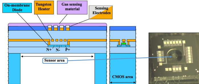
Figure 1: Cross-section and top view of the SOI sensing platform with embedded electrodes, heater and diode.
