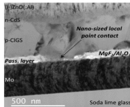
Figure 1: TEM cross-section of a rear surface passivated  $\text{Cu}(\text{In,Ga})\text{Se}_2$  solar cell [1].
