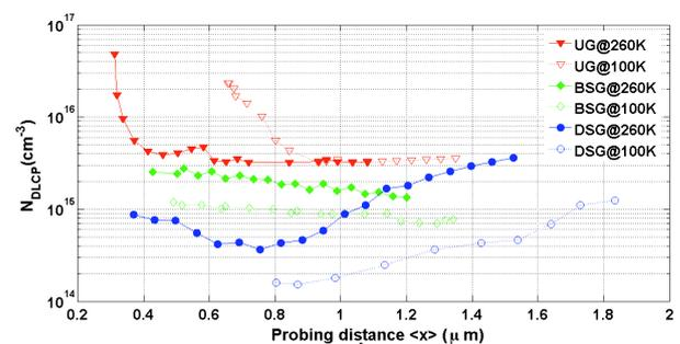
Figure 2: Deep-level-capacitance-profiling (DLCP) of  $\text{Cu}(\text{In,Ga})\text{Se}_2$  solar cells [2].
