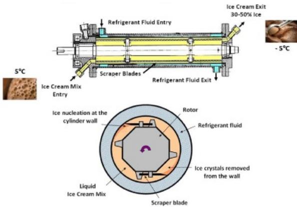
Figure 1: Schematic view of the ice cream crystallizer.
