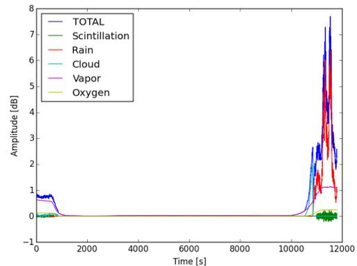
Figure 1: Simulation of time series of total attenuation encountered during a flight.
