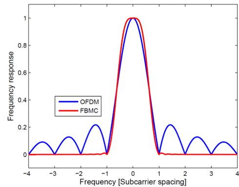
Figure 1: Frequency response of the prototype filters in OFDM and FBMC multicarrier modulations.
