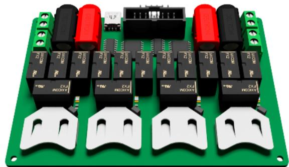
Figure 2: 3D model of the adaptive battery management system printed circuit board designed for four coin/pouch cells.
