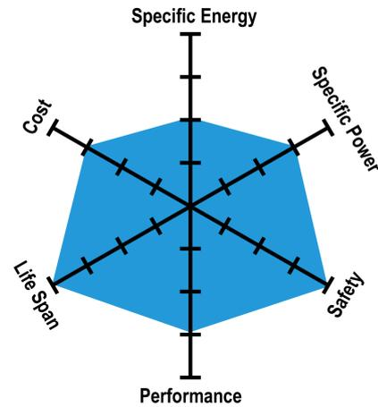
Figure 1: Lithium iron phosphate battery characteristics.
