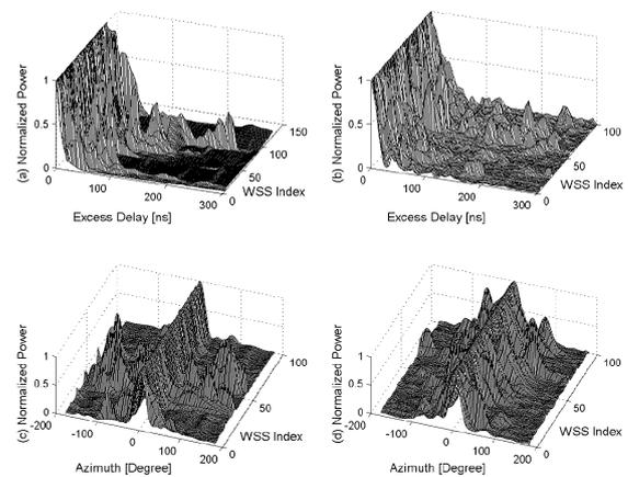
Figure 1: Comparison of measured (left) and simulated (right) power-delay and power-angular profiles in suburban environments.
