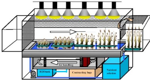
Figure 1: Schematic view of the greenhouse.
