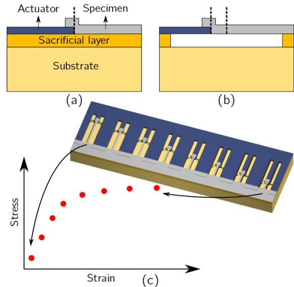
**Figure 1: Principle of lab-on-chip concept: side view showing the different layers (a) before and (b) after etching of sacrificial layer, and (c) set of structures for extraction of full stress-strain curve.**
