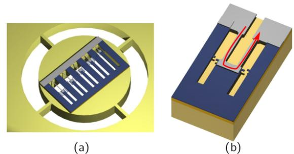
**Figure 2: Designs of two extensions of the lab-on-chip concept : (a) Backetching for TEM analysis and (b) design of an elementary test structure for electro-mechanical characterization.**
