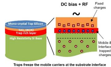
Figure 1: Cross-section of a trap-rich SOI substrate with its carrier distribution at equilibrium.
