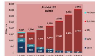
Figure 3: Rapid adoption of trap-rich SOI substrate for RF switches.
