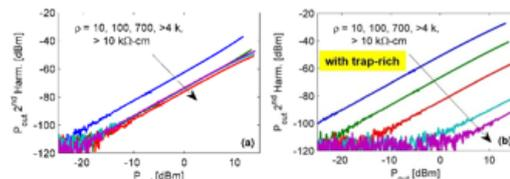
Figure 2: - Measured second harmonic output power of a 2,146-μm-long CPW line on n-type Si with different resistivities (a) without and (b) with a trap-rich polysilicon layer.
